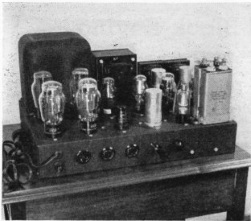
This power supply chassis contains the three supplies shown in Figs. 6, 7 and 8. Right — bottom view of the power supply chassis.
