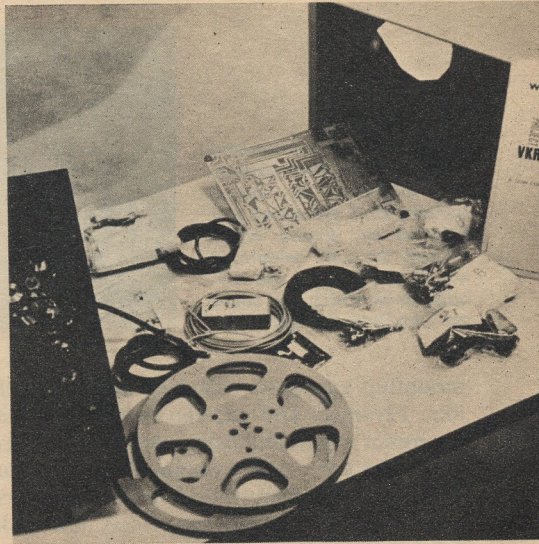
Kit consists of basic tape-transport mechanism and necessary record and replay electronics. Most components mount on single printed-circuit board.
